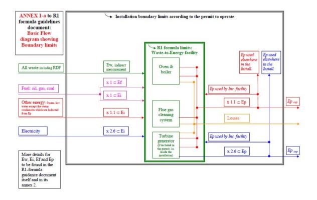
Figure 2:Distinction between R1 system boundary and permit boundary for MSWI<br/>(Source: CEWEP-ESWET-FEAD Proposal for a Guideline for the use of the R1 energy efficiency<br/>formula for incineration facilities dedicated to the processing of Municipal Solid Waste (Waste<br/>Framework Directive 2008/98/EC, Annex II, R1-formula), 30 Nov 2009.
