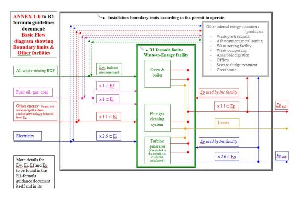
Figure 3: Other internal uses excluded from the R1 system boundary
